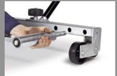
The rollers have three positions each side for different wheels sizes.
